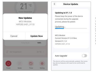
XVELTRON Smart Heater upgrades firmware online. Manufacturers may upgrad@irmware to modify features or improve performant@memew firmware is released, we will notify you that there is new firmware that needs to be installed through the Smart Life app. If you agree and press the upgrade button, the new firmware will be automatically downloaded and upgraded, and the heater will restart with the newly upgraded firmware
